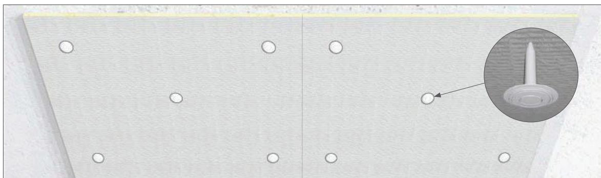
Figure 1.4. Insulation fastener
