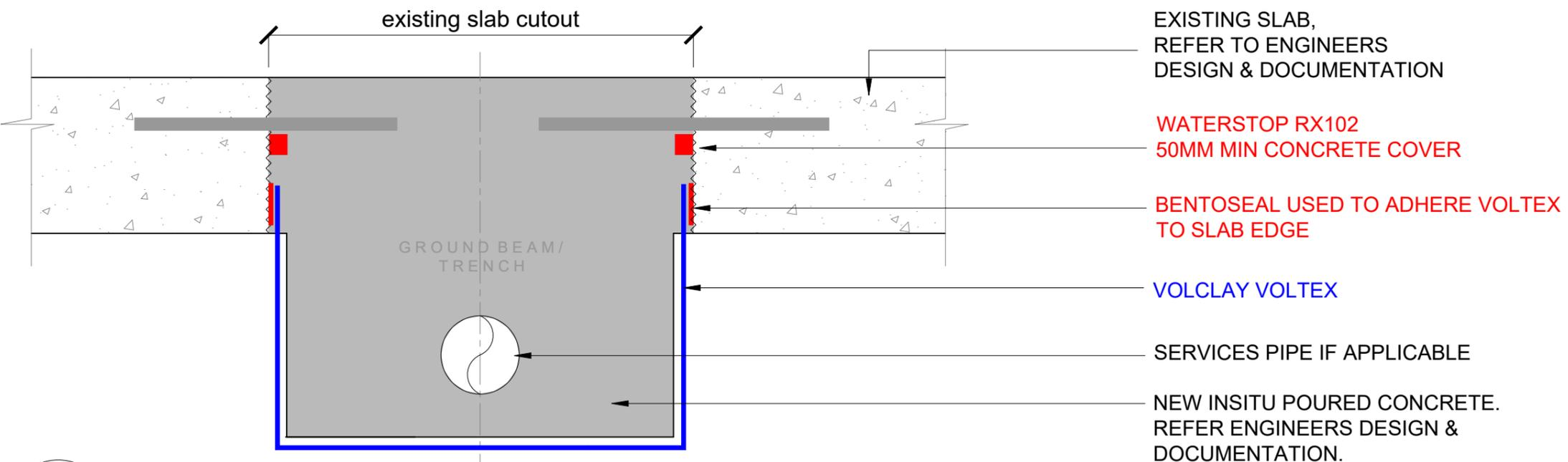
**2** NEW BEAM / SERVICES TRENCH TO EXISTING SLAB
