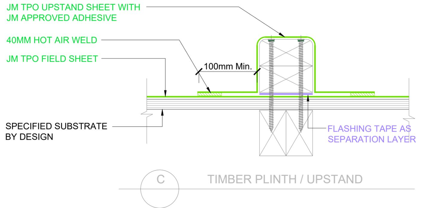
Although ALLCO do not recommend fixing posts or plant through the top of Membrane roofs or decks if this is required then use a plinth detail provides the fixing by other trades are kept off the main deck flood area. ALLCO recommend that all plantwork fixings are kept independent of the membrane roof ideally through vertical surfaces such as parapets.
