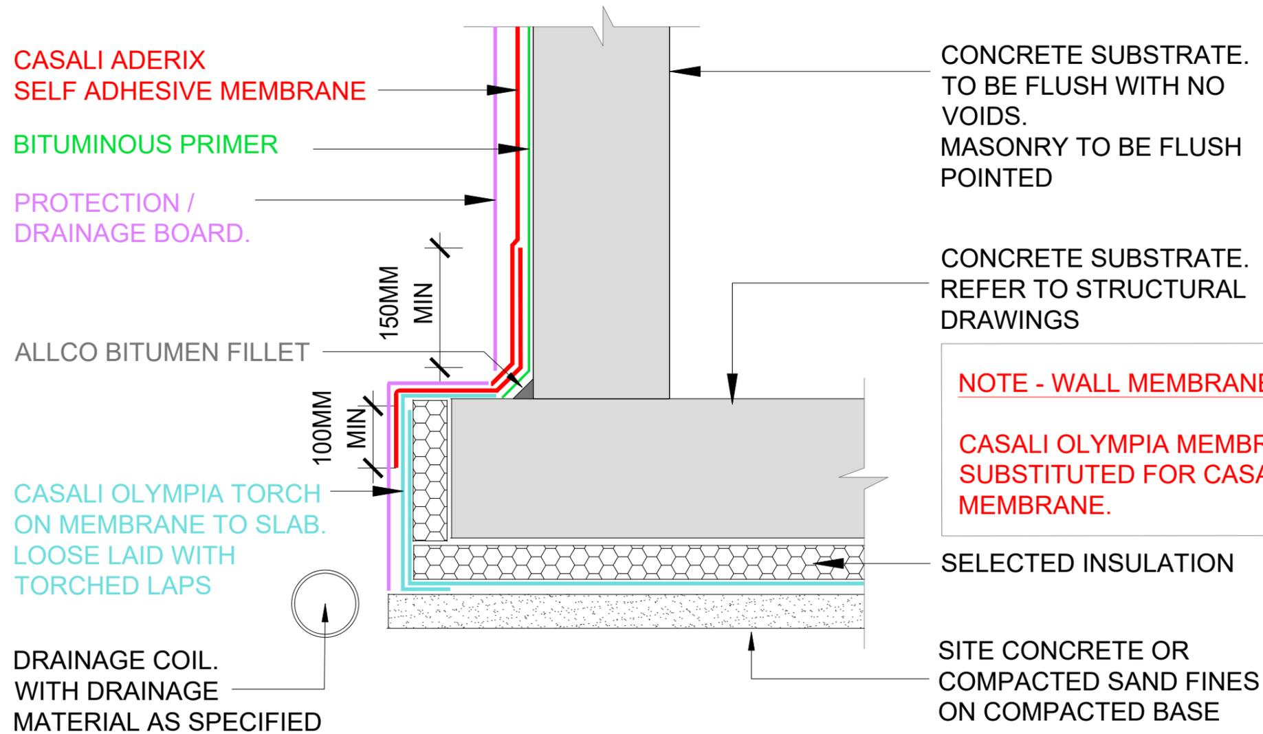
1 RETAINING WALL / HEELED FOOTING JUNCTION TO INSULATED SLAB
