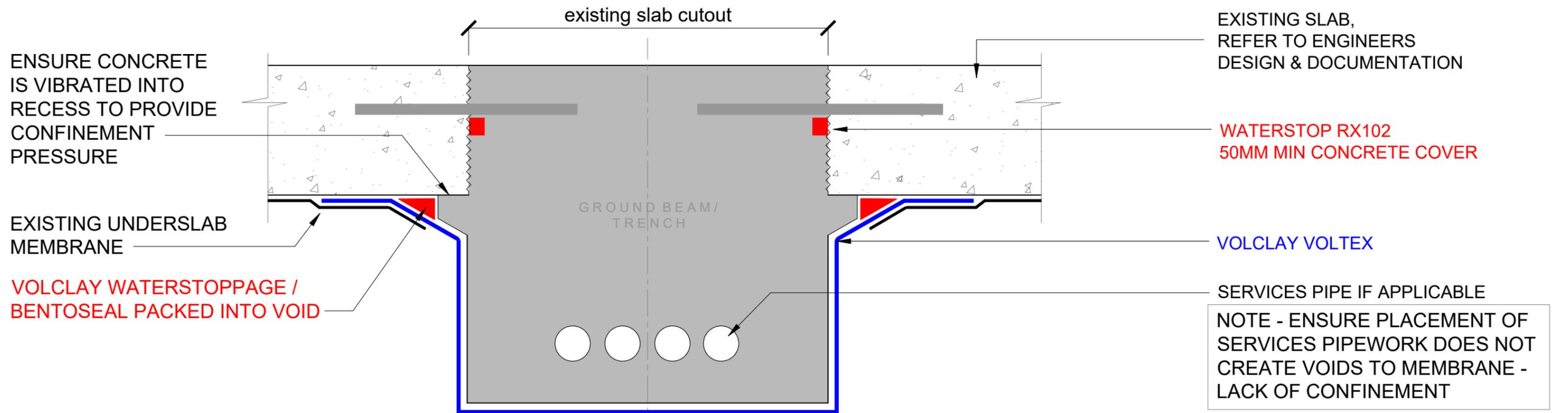
**1** NEW BEAM / SERVICES TRENCH TO EXISTING SLAB
