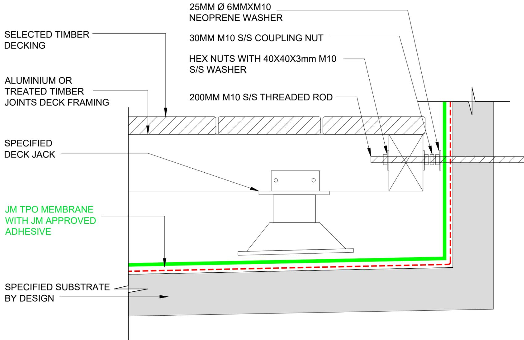
1 UPSTAND DETAIL - DECK FRAMING EDGE FIXING
