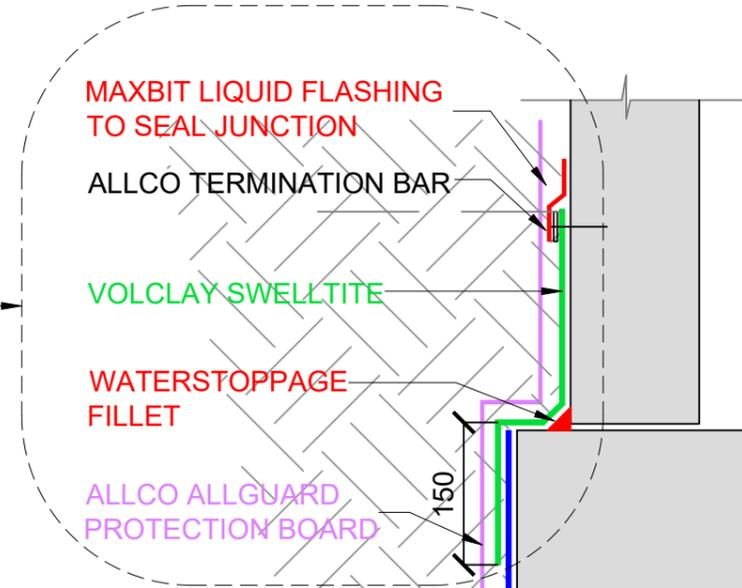
STRUCTURAL CONCRETE CAPPING AND PILE. REFER ENGINEERS DESIGN & DOCUMENTATION.
