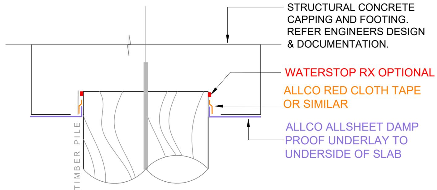
1 FOUNDATION DETAIL - TIMBER PILE / CAPPING BEAM DPM
