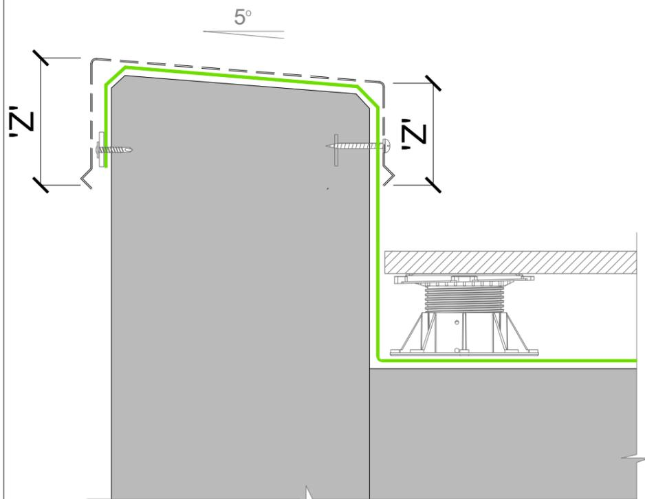
1 JM TPO - GREEN ROOF PARAPET - PAVED AREA
