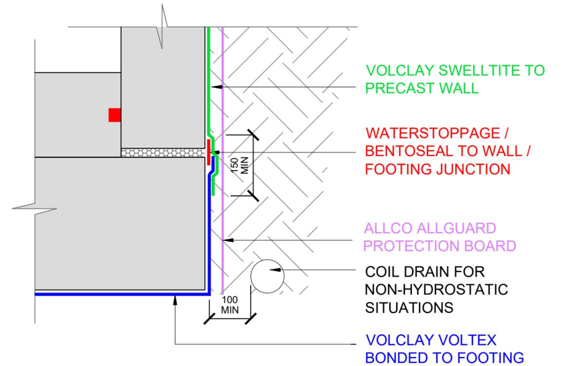
**1** FLUSH FOOTING / WALL - BONDED VOLTEX TO PC PANEL
