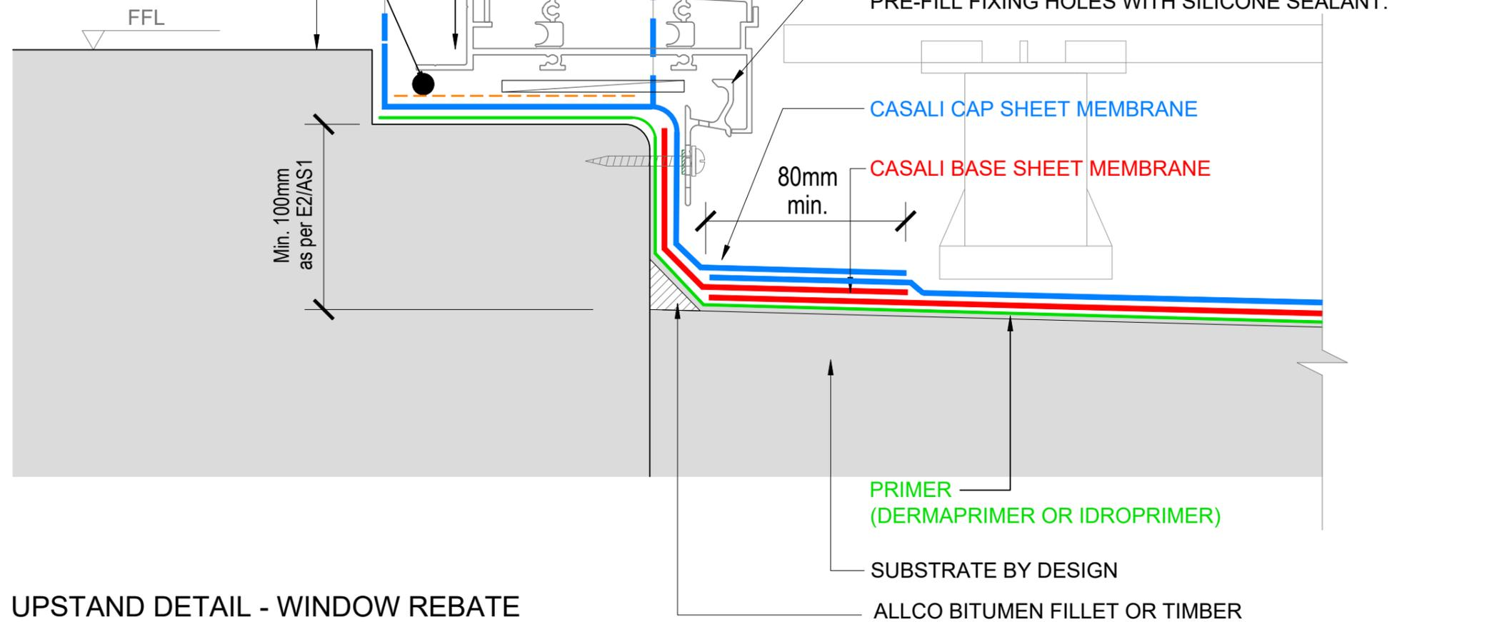
FINISH MEMBRANE 100MM MIN. UP FRAMING AT ENDS. WIDTH TO SUIT JOINERY AND CLADDING. REFER E2/AS1 FIG62(B)(D)
