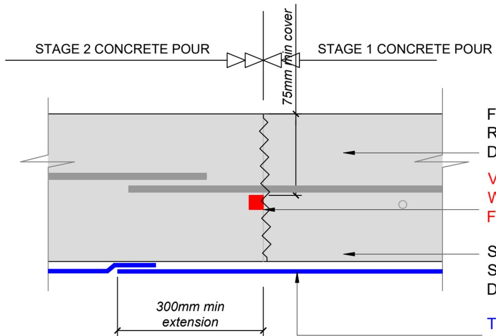
FLOOR SLAB REINFORCEMENT,
