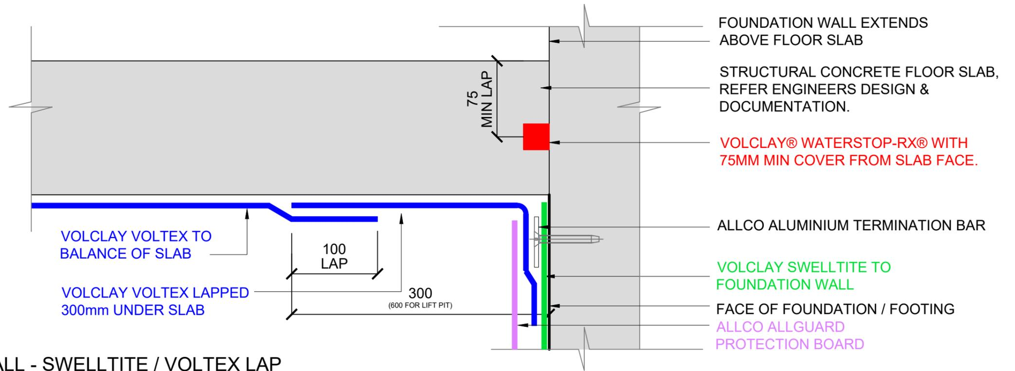
**2** FLOOR SLAB TO WALL - SWELLTITE / VOLTEX LAP
