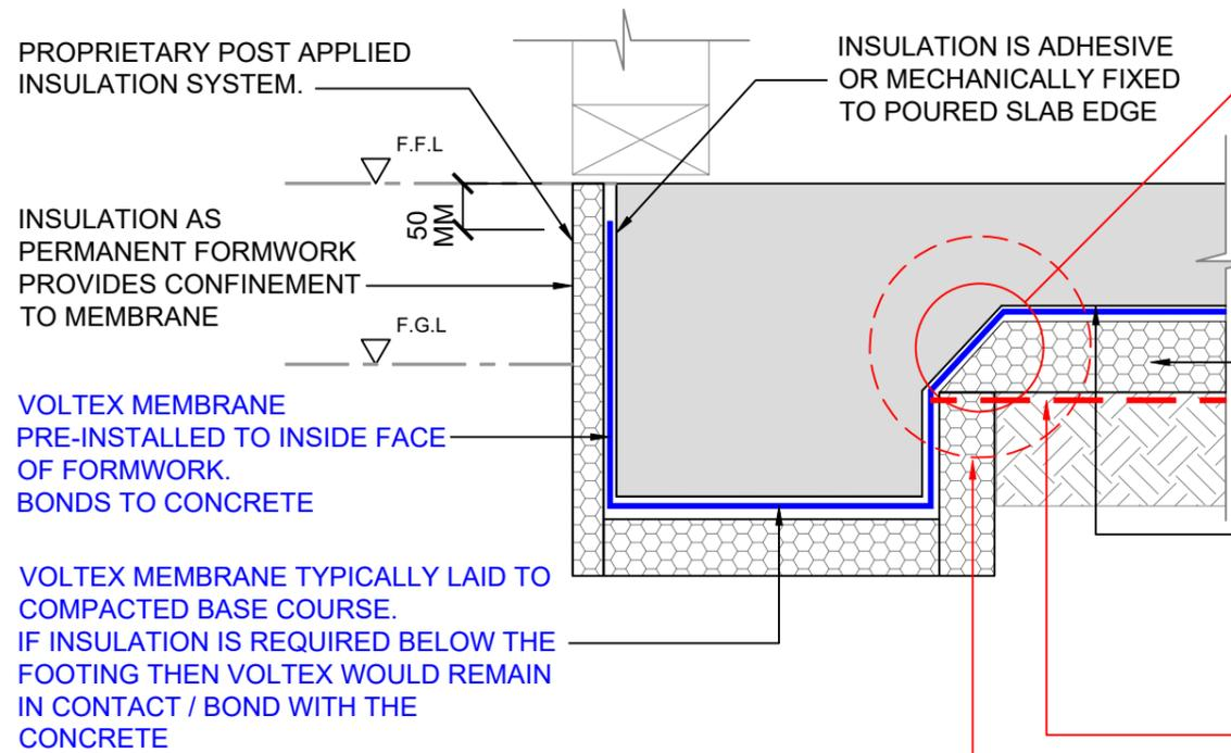
ALLOW TO PLACE HAUNCHING TO ENDS OF INSULATION PANELS OR CHAMFER TO MINIMISE MOVEMENT AND FILL VOIDS TO FOOTING / SLAB TRANSITION
